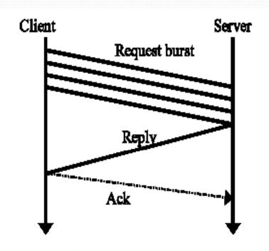
**Figure 4.4.** RPC using a burst protocol; here the reply is sent soon enough so that an acknowledgement to the burst is not needed.
